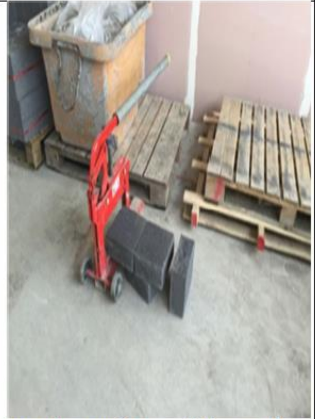
Good practice – Using a low energy solution such as a block splitter (HSA, IE)
